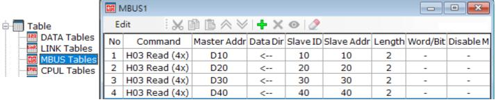
**4.** After completing previous 3 steps, this Master PLC with the MBUS table and instruction will become a Client. Then, the card will transfer the Modbus RTU command to the Modbus TCP/UDP IP protocol to access data in Slave devices. In addition, if the Master
