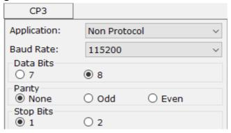
**3.** Thus, when the Client sends a packet through the Ethernet IP and Port #2000 to this RS Server mode card, will be converted to the PLC's CP3 serial communication port. Then, the PLC could use the RS instruction to analyze the data.
