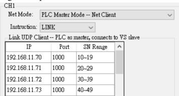
2. Open the Ladder Master S to edit the Master PLC's project, under the menu bar's [Project] – [COM Port Setup...] to let the PLC's CP2 become "VS Computer Link Master", Baud Rate 115200 (should match with card's CH1).
