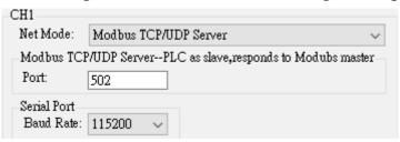
2. Open the Ladder Master S to edit a PLC project, under the menu bar's [Project] – [COM Port Setup...] to let the PLC's CP2 become "MODBUS Slave", Baud Rate 115200 (should match with card's CH1) and the Station Number use default #1. Then, use a Mini USB cable to load this project to the PLC.
