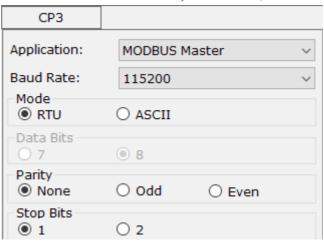
**3.** Under the [Project] – [MBUS Tables] to edit a table. Finish the table and add the MBUS instruction in the program. Then, use a Mini USB cable to load this project to the PLC.
