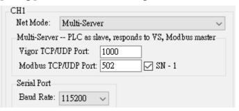
2. Open the Ladder Master S to edit a PLC project, under the menu bar's [Project] – [COM Port Setup...] to let the PLC's CP2 become "VS Computer Link Slave", Baud Rate 115200 (should match with card's CH1) and the Station Number use default #0. Then, use a Mini USB cable to load this project to the PLC.
