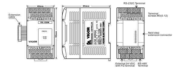
POWER LED : Lt when 5 VDC power supplied from the PLC.
