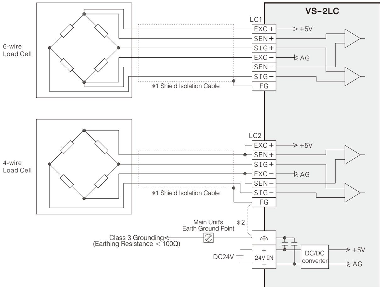
\*1 : Please use the shield isolation cable for the load cell. Must keep the signal cable away from any power line (including the power of motor, valve or contactor) to prevent external interference or module damage.
