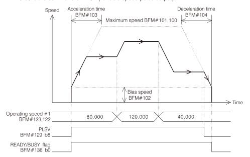
When the axis is for to use the PLSV (BFM#129 b8 = ON) function, it will use the value of operating speed #1 (BFM#123, 122) to generate pulses. Give a positive operating speed will have a forward movement, on the other hand, a negative operating speed will move backward.
