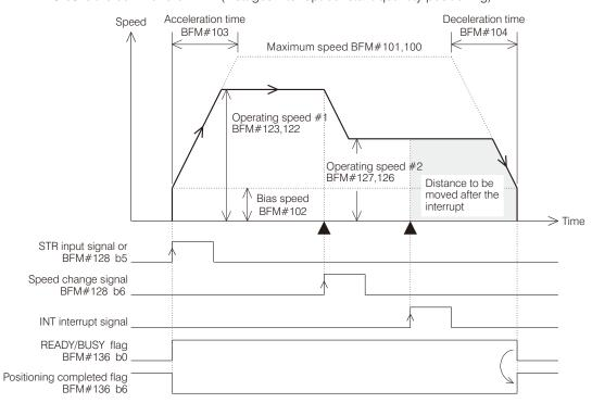
When the axis is for to use the DV2I (BFM#129 b6 = ON) function and the start signal is turned from OFF to ON, its output pulse string will be executed as above. Distance to be moved after the interrupt = Target position #1 (BFM#121, 120)
