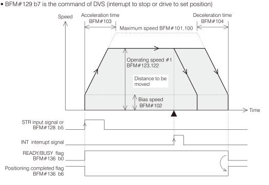
When the axis is for to use the DVS (BFM#129 b7 = ON) function and the start signal is turned from OFF to ON, its output pulse string will be executed as above.
