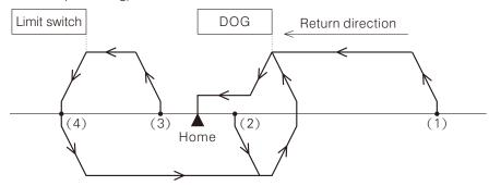
The diagram above illustrates the different actions from the starting points (1) $\sim$ (4) to complete the home positioning.
