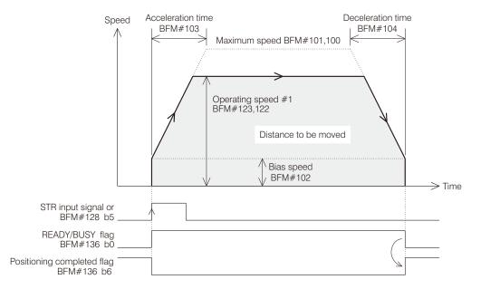
When the axis is for to use the DRV (BFM#129 b3 = ON) function and the start signal is turned from OFF to ON, its output pulse string will be executed as above.
