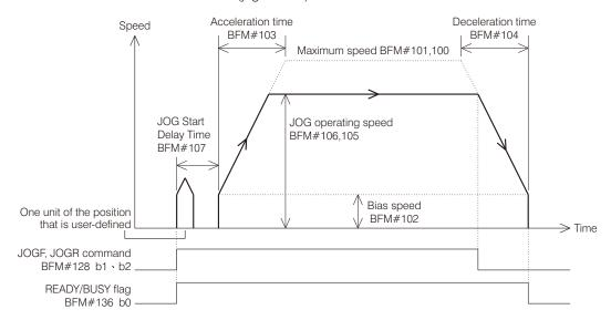
When the axis is for to use the JOGF (BFM#129 b1 = ON) or JOGR (BFM#129 b2 = ON) function, its output pulse string will be executed as above. During the operation, could change the value of BFM#106, 105 or BFM#114 to modify the real operating speed.
