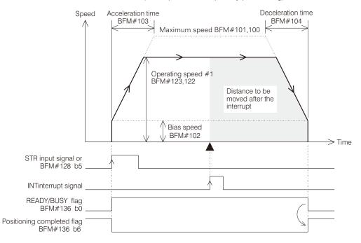
When the axis is for to use the DVIT (BFM#129 b5 = ON) function and the start signal is turned from OFF to ON, its output pulse string will be executed as above.
