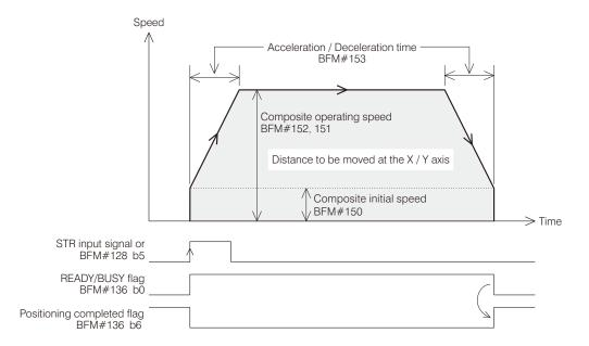
When the paired axes are for to use the LI (BFM#129 b10 = ON) function and the start signal is turned from OFF to ON, their output pulse strings will be executed as above.
