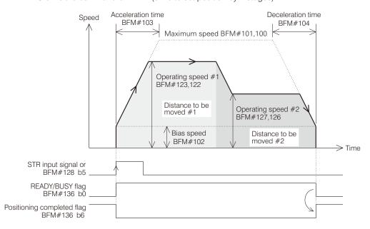
When the axis is for to use the DRV2 (BFM#129 b4 = ON) function and the start signal is turned from OFF to ON, its output pulse string will be executed as above.
