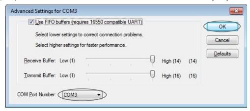
4 After finish those settings, the computer's USB port could connect with a **Lyicor** PLC's CP1 via this adapter.
