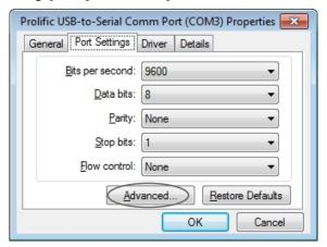
In the [Advanced Settings] there is the [COM Port Number:] could be selected. Choose an unoccupied port between COM3 ~ COM16 for the Ladder Master then click the [OK] to exit.
